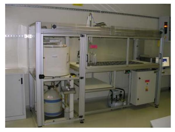
The SCS is designed in such a way that it can make use of existing lead shields and detectors. The control is done via an industrial PLC that is connected to a standard PC using windows as software platform.
